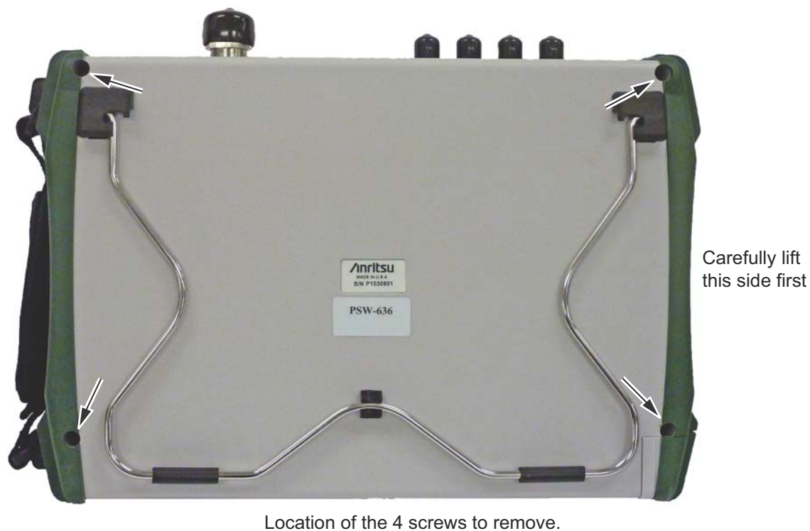
Figure 5-2. Remove the Four Screws
